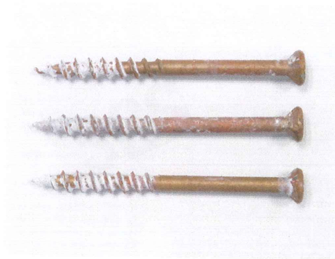
Specimen Name: Aegis Coating Screw(AS-7573) After 1000 Hours Test
